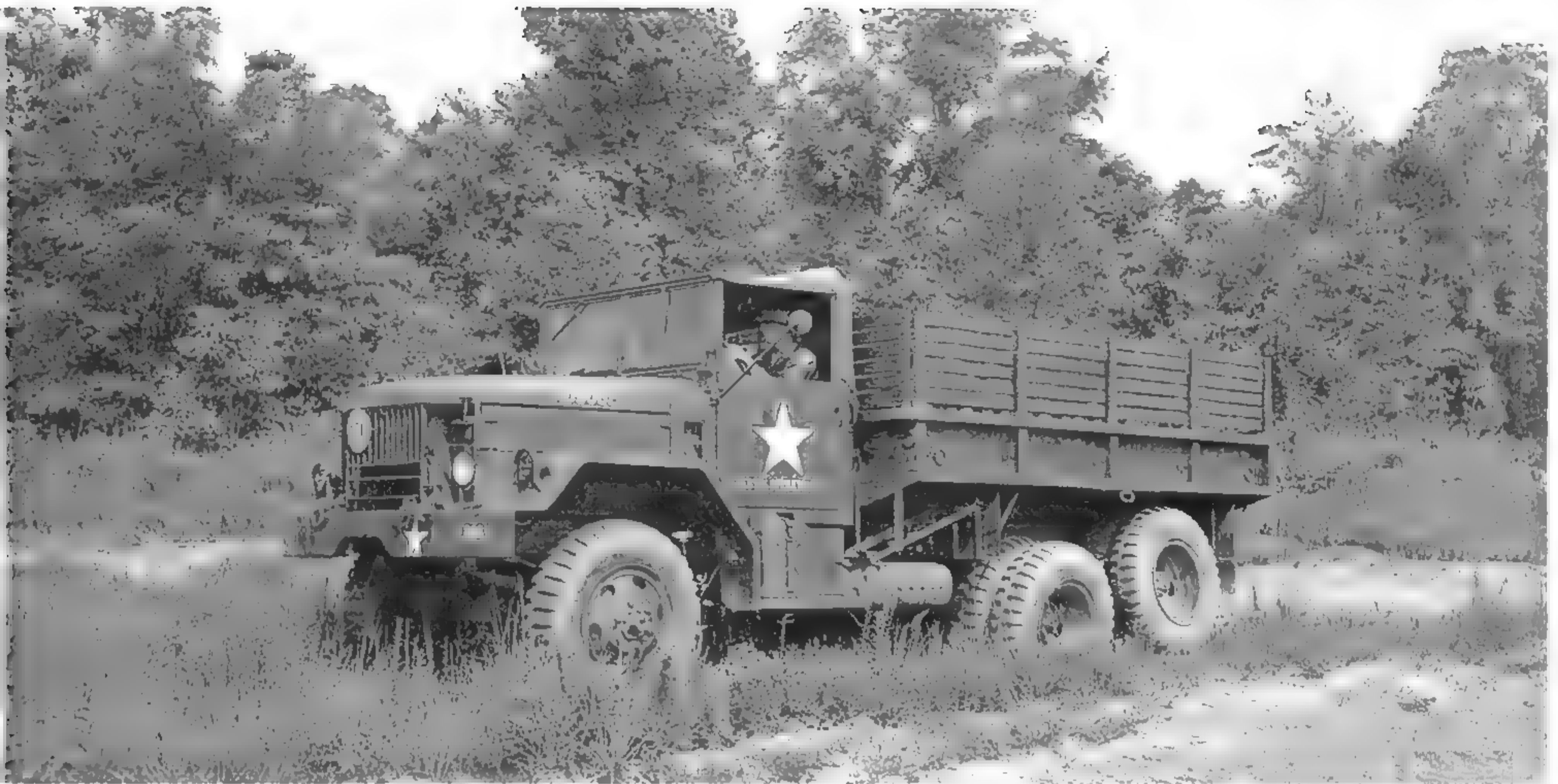
The M35A1, although resembling the M35, was greatly improved with the introduction of the LDS-427-2 Multifuel engine and overdrive transmission. This photo of an M35A1 on a test course shows the rear suspension travel. (U.S. Army photo)
